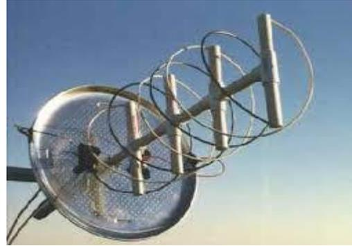
Figure 15: Long Helical Antenna [12]
