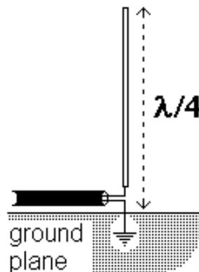
Figure 13: Quarter-dipole antenna [1]
