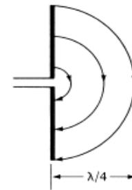
Figure 2: Electric Field at  $t = T/4$  [1]
