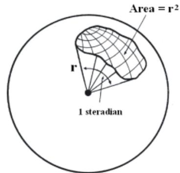
Figure 7: Steradian: The Solid Angle [8]
