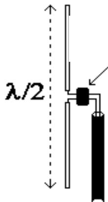
Figure 12: Half-dipole antenna [1]
