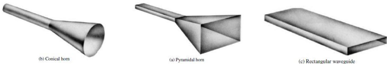
Figure 10: Aperture antennas [1]
