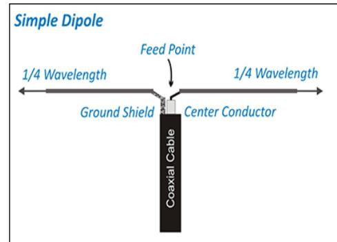
Figure 1: Half Wave Dipole Antenna [4]
