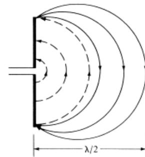
Figure 3: Electric Field at  $t = T/2$  [1]
