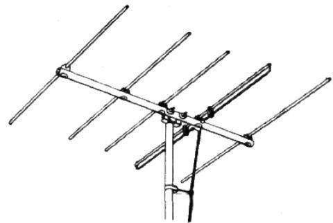
Figure 14: Yagi-Uda Array Antenna [10]
