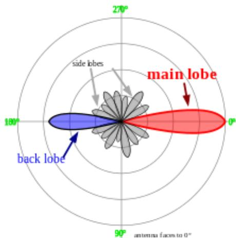
Figure 5: Two-Dimensional Radiation Pattern [6]
